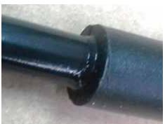
**11.** Leave the completed joint to COOL for 5 minutes to ensure that the glue seal isn't damaged. Once cooled, momentarily power the light to confirm that the connection is sound.
