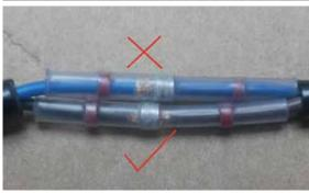
7. Using a heat gun on Medium to High heat, gently heat the centre of the solder splices until the solder ball melts and runs into the wire. Take care to only heat around the solder ball as excess heat can damage the cable. Check that the red seals next to the solder balls have also melted.
