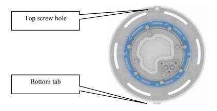
**c.** Insert the protruding tab into the slot at the bottom of the mounting plate by holding the light at an angle to the wall, then seat the light into the mounting plate. Reinsert the original retaining screw to hold the light in position. Do not over-tighten; using power tools may cause damage. Before filling the pool check the light is functioning by switching it on for a few seconds.
