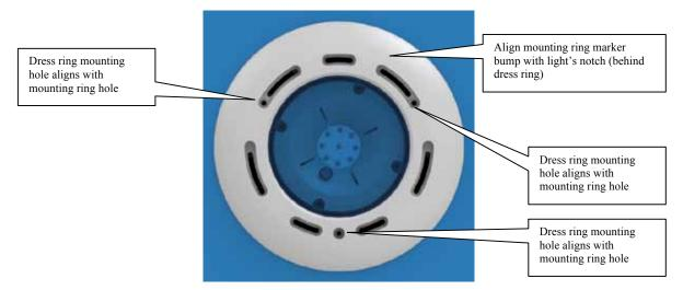
**b.** Using the three screws in kit 13529, attach the light and dress ring to the niche using a manual screw driver. Do not over-tighten; using power tools may cause damage. Before filling the pool check the light is functioning by switching it on for a few seconds.
