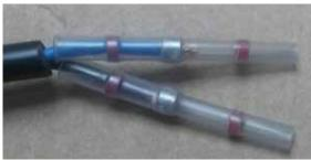
**6.** Slide the wires from the new cable into the solder splices and position each splice so that the silver coloured solder ball is positioned over where the 2 wires join.
