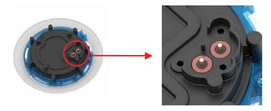
**3.** Align the plug with the socket on the light and use the three screws from kit 20350 to attach the plug securely to the light. Tighten these screws by hand only; do not use a power tool.
